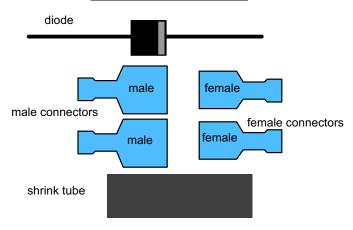
**STEP 1:** Trim each lead on the diode to 3/8" long, as shown.
